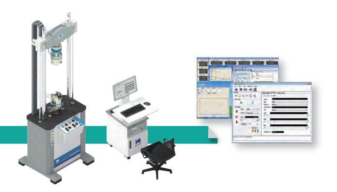
The actuating cylinder with test load of ± 10 to ± 3000kN can be selected The upper crossbeam can be The standard configuration is adjusted, and hydraulic crossbeam the force sensor is located on fixing and lifting hydraulic cylinder
